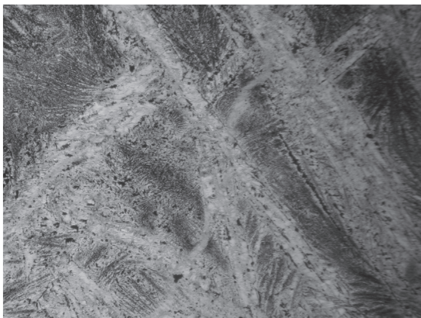
Fig. 2. Photomicrograph: enlargement of Fig. 1 (field of view 0.5 mm) shows several generations of spinifex-textured quench crystals, including radiating fans of pyroxene (now replaced by serpentine) and delicate opaque (black) needles and trains of granular chromite.
